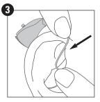
**Step 3:** While holding the RU in place in the ear canal with your thumb or index finger; carefully place the hearing instrument body over the top of
