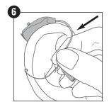
*Caution:* When removing the RU, do NOT pull with the body of the hearing instrument as this may damage the connection.
