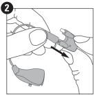
**Step 3:** Remove the used filter from the hearing aid as displayed in illustration 3.
