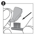
See illustration 1, showing proper method. Also brush the microphone port as shown in illustration 2. If the hearing instrument is weak or not working, you may need to replace the wax guard as outlined in this manual. Inspect the RU and wax guard daily for any visible damage. If any damage has occurred, or the wax guard comes off inside the ear, contact your hearing care professional for immediate help.
